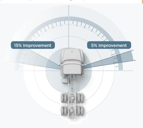
The shaded areas represent how indirect visibility has been optimized by reshaping the doors and side windows, and repositioning the cab mirrors so drivers turn their heads 15% less on the driver side and 5% less on the passenger side. This increased visibility reduces driver stress and neck strain to enhance productivity.
