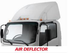
To help maximize fuel efficiency, the customdesigned Isuzu air deflector directs air over the top and around the sides of body to reduce drag.
