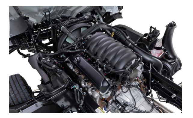
The rigorous driving demands of medium-duty trucks require a durable powertrain. Integral to this is a cast-iron block specifically designed for heavy-duty use with channels incorporated for jet-spray piston cooling to help the engine run cooler and *more efficiently*. Additionally, an aluminum head design incorporates direct injection, variable valve timing, and an air intake humidity sensor that manages the 6.6-liter
