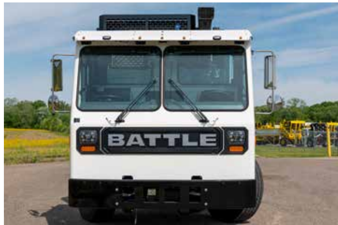
82" cab width engineered to be 12" narrower than our standard chassis for tight applications
